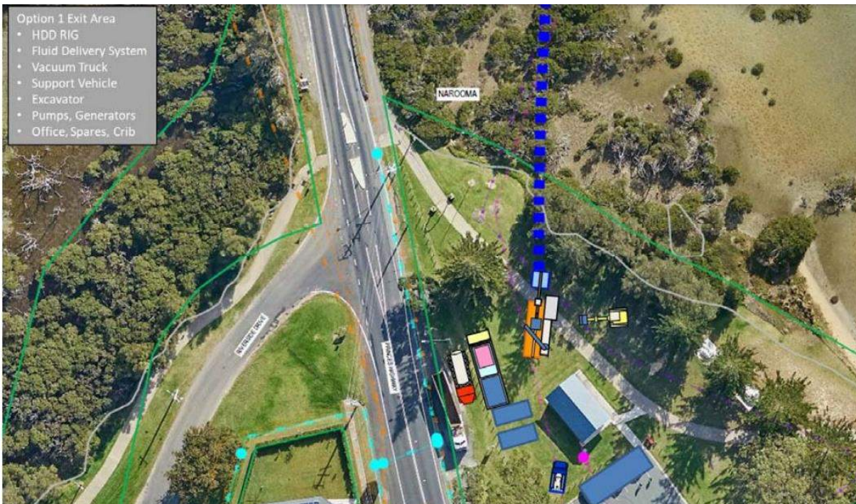
Figure 3.4 Exit site (Ken Rose Park) showing proposed locations of ancillary facilities
