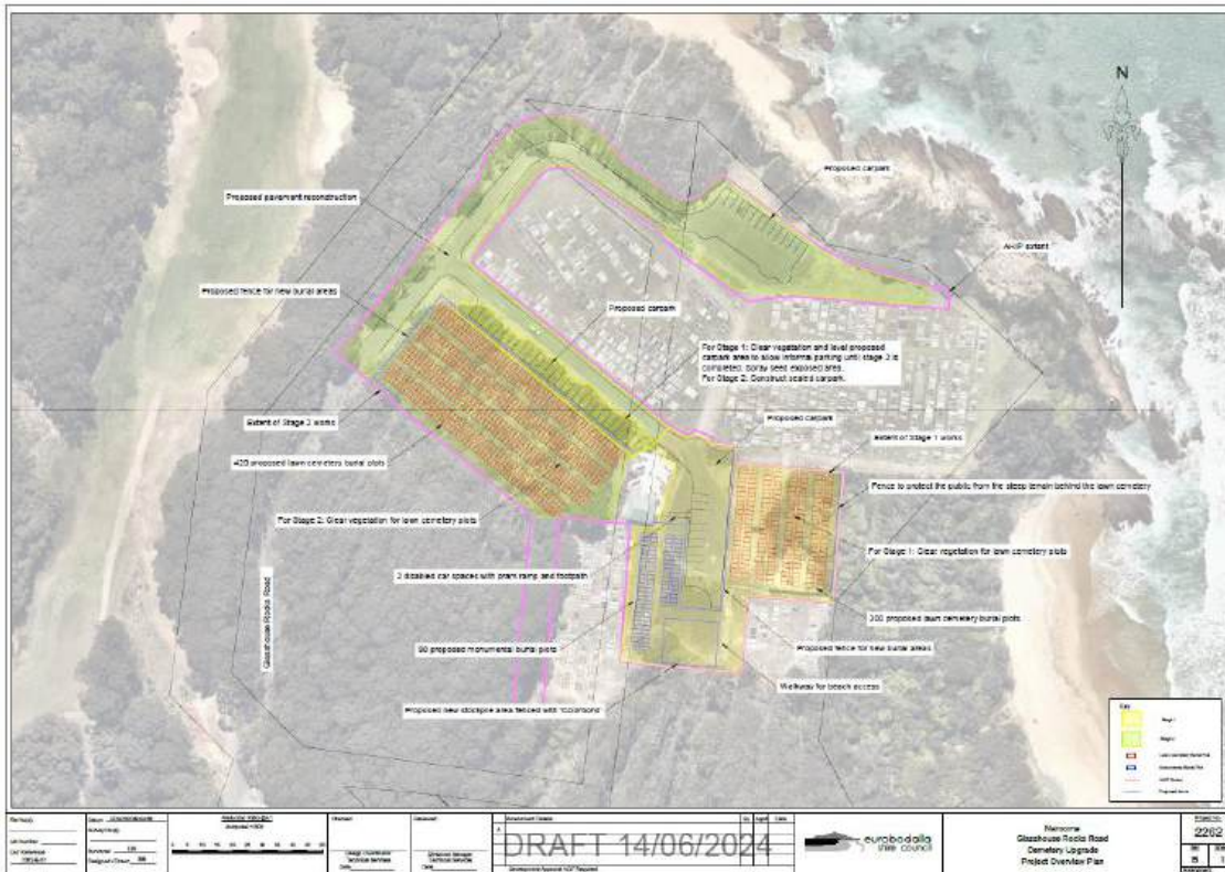
Figure 2. Scope of works for expansion of The Narooma Cemetery under the current master plan.
